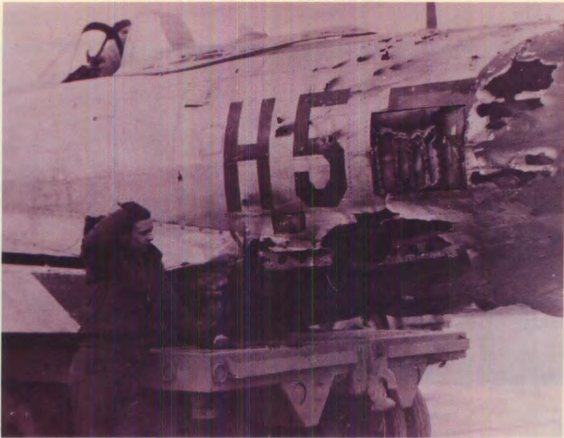
His crash-landed JUG ready for the salvage dump, Ist Lt. Hoyt Bengé examines the damage resulting from a direct hit by a 88mm shell during a dive-bombing mission over Germany. Despite the severe damage, Lt. Bengé flew the plane back to base and landed unhurt.
